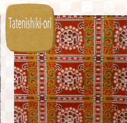
Patterns are woven with warps of 3 or more colors and wefts with 2 or more colors.
